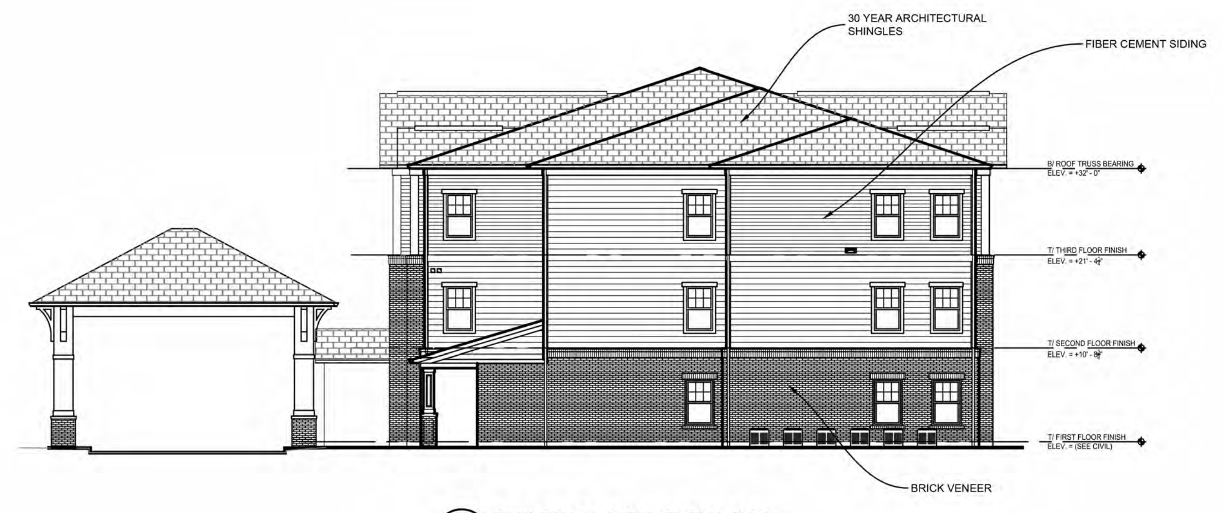
2 BUILDING - SIDE ELEVATION 3/32" = 1'-0"
